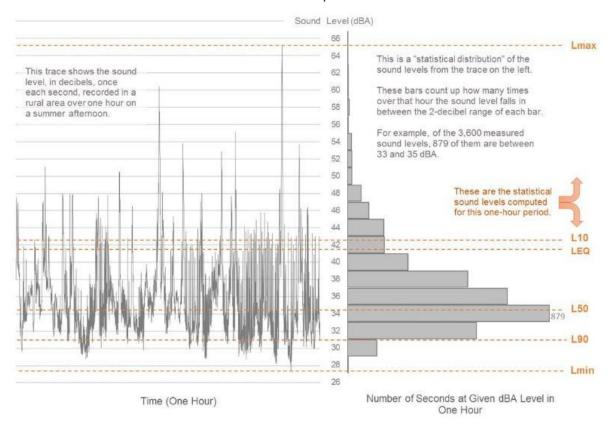
FIGURE 33: EXAMPLE OF DESCRIPTIVE TERMS OF SOUND MEASUREMENT OVER TIME
