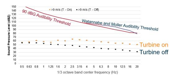
FIGURE 5: INFRASOUND FROM A WIND TURBINE AT 350 METERS (1,148 FEET) COMPARED WITH PERCEPTION THESHOLDS
