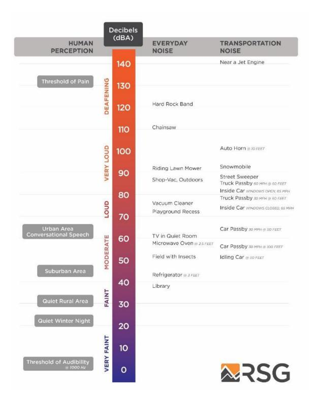
FIGURE 32: A SCALE OF SOUND PRESSURE LEVELS FOR TYPICAL SOUND SOURCES
