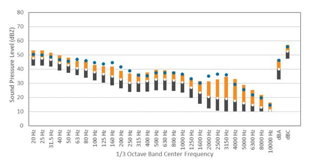
FIGURE 28: OFFSITE E MONITOR - 1/3 OCTAVE BAND AND OVERALL STATISTICAL SOUND LEVELS (FOR PERIODS WITH A 9 m/s WIND SPEED AT 89-METER (292-FOOT) HEIGHT)
