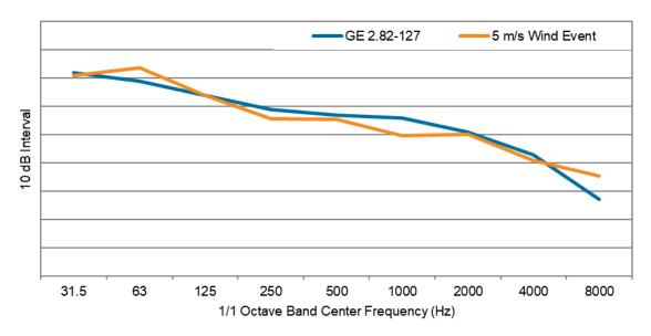
FIGURE 4: COMPARISON OF NORMALIZED FREQUENCY SPECTRA FROM THE WIND AND THE GE 2.82-1276
