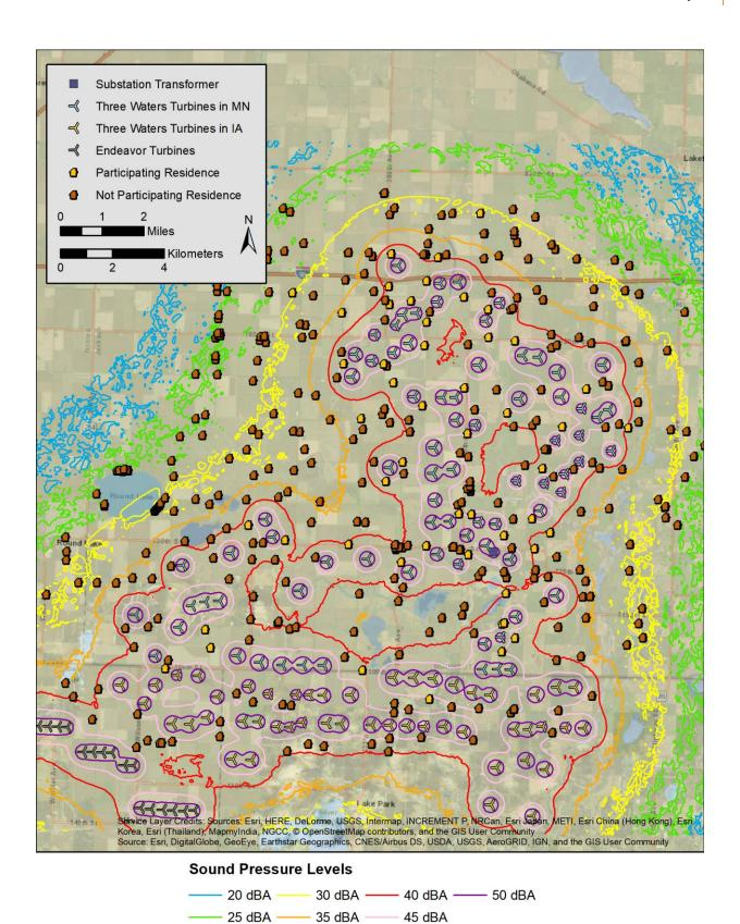
FIGURE 31: SOUND PROPAGATION MODEL RESULTS
