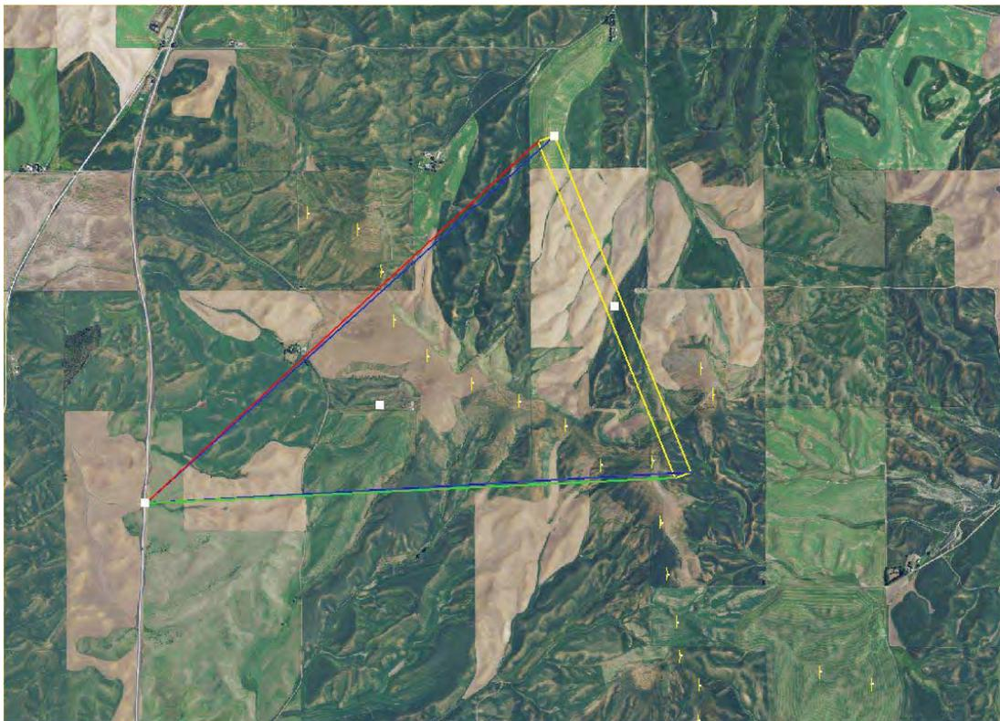
**Exhibit 2:** Step 2 - Aerial orthographic photo view cone with photo location and turbines locations.
