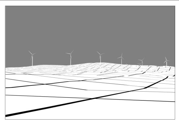
**Exhibit 3**: Step 3 - Digital overlay of terrain and turbines to allow alignment with photograph.
