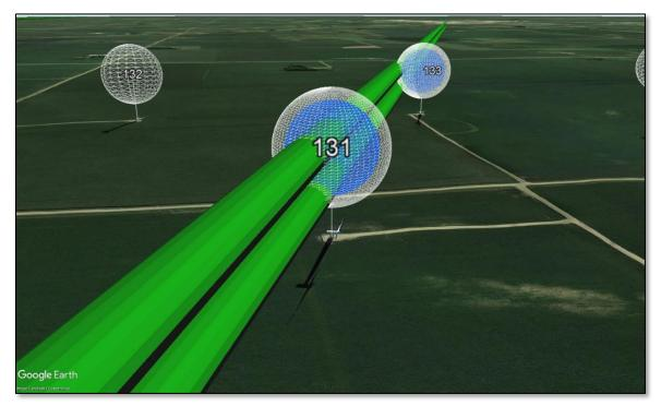
Figure 9: T131 and T133 existing rotor diameter (blue) and increased rotor diameter (white) rotor-swept spheres intersecting the WQAU442/WQOZ385 Fresnel zones
