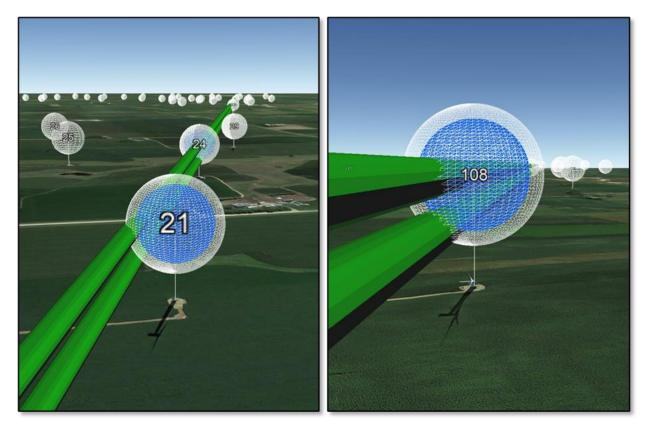
Figure 7: T21, T24 (left), and T108 (right) existing rotor diameter (blue) and increased rotor diameter (white) rotor-swept spheres intersecting the WQAU442/WQOZ385 Fresnel zones
