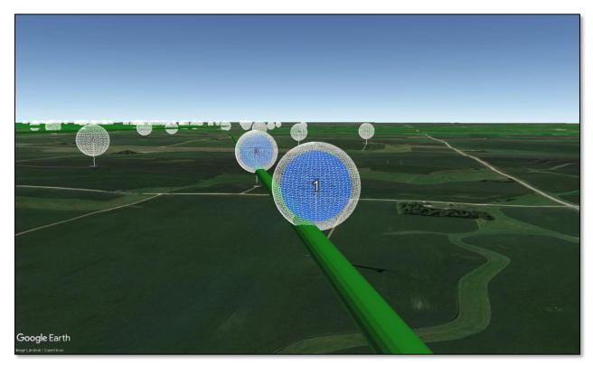
Figure 4: T1 and T3 existing rotor diameter (blue) and increased rotor diameter (white) rotor-swept spheres intersecting the WQXT655/WQXT661 Fresnel zone
