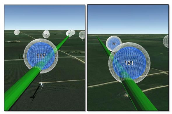
Figure 6: T117 (left) and T131 (right) existing rotor diameter (blue) and increased rotor diameter (white) rotor-swept spheres intersecting the WQXT661/WRCK732 Fresnel zone
