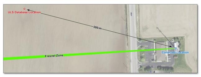
Figure 3: Example of using aerial imagery to correct erroneous ULS database antenna location
