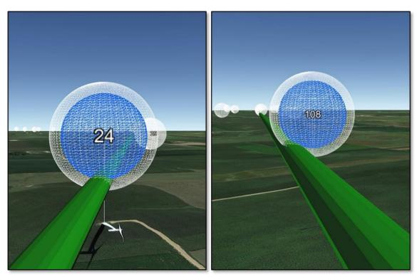
Figure 5: T24 (left) and T108 (right) existing rotor diameter (blue) and increased rotor diameter (white) rotor-swept spheres intersecting the WQXT661/WRCK732 Fresnel zone
