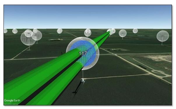
Figure 8: T117 existing rotor diameter (blue) and increased rotor diameter (white) rotor-swept spheres intersecting the WQAU442/WQOZ385 Fresnel zones
